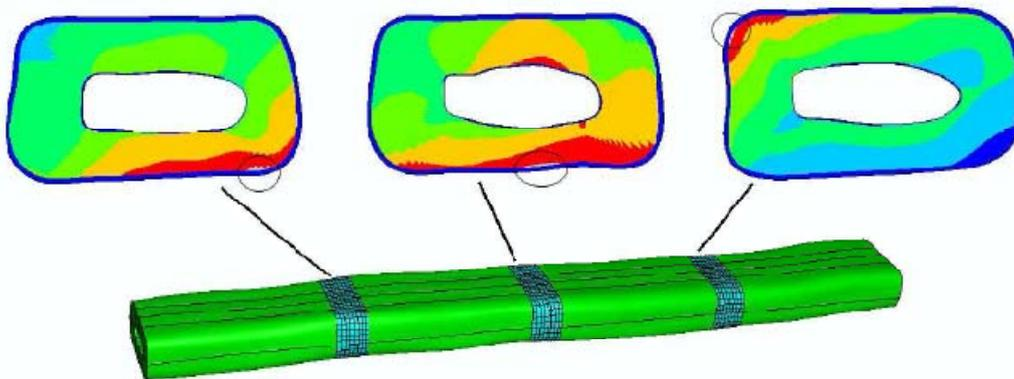
Figure 1: Three dimensional stress analysis and comparison with a Tsai-Hill failure in tensile loading of a geometrically well-characterized wood fibre. Hot-spots indicate zones of probable failure.
