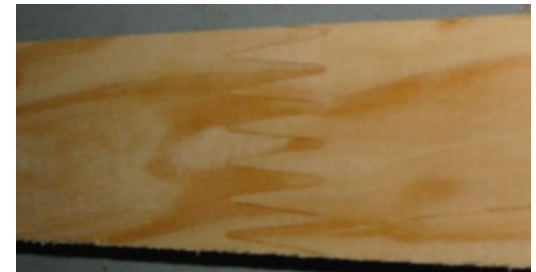
Picture of the green Finger joint
