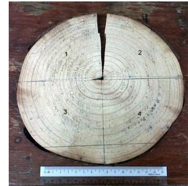
On the left, the intact disc shows less variation between radial and tangential swelling than on the right where a crack has developed at T1.
