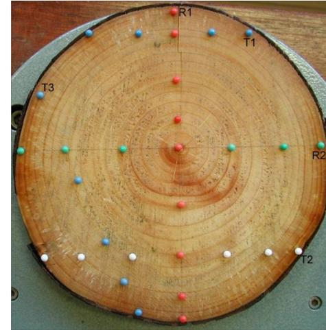
The same disc was then quarter sawn and the experiment repeated to assess the impact of the release of stresses within the disc.
