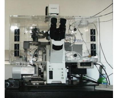
time-resolved scanning acoustic microscope, SASAM (P.V. Zinin)
