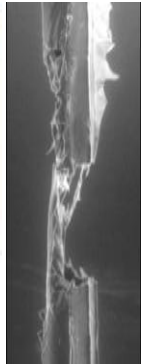
Micro-tensile testing stage and fiber fracture zone ( Eder et al. 07 )
