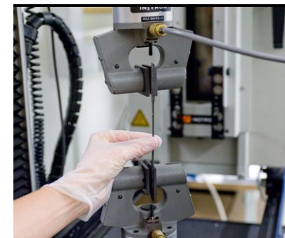
Tensile testing of Vasa material ( Bjurhager, Kristensson '10 )
